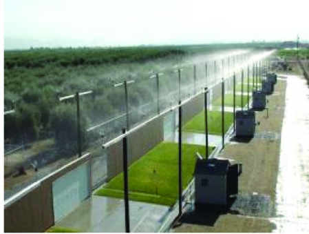
(b) Rainfall simulator on cross beams
